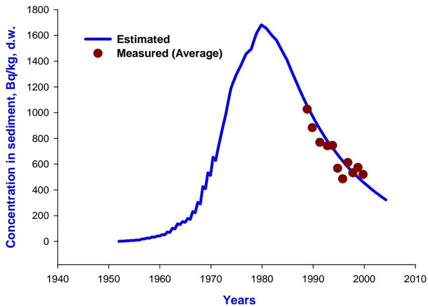
Figure 5.4. Comparison between model simulation and measurements for the Cumbrian waters for  $^{239,240}\text{Pu}$  discharge into the Irish Sea
