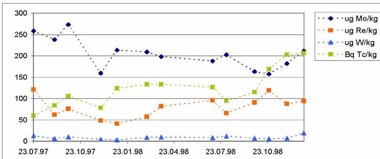
Figure 8. ICP-MS determination of Tc, Re, W and Mo in a series of seaweed collected from Northern Norway
