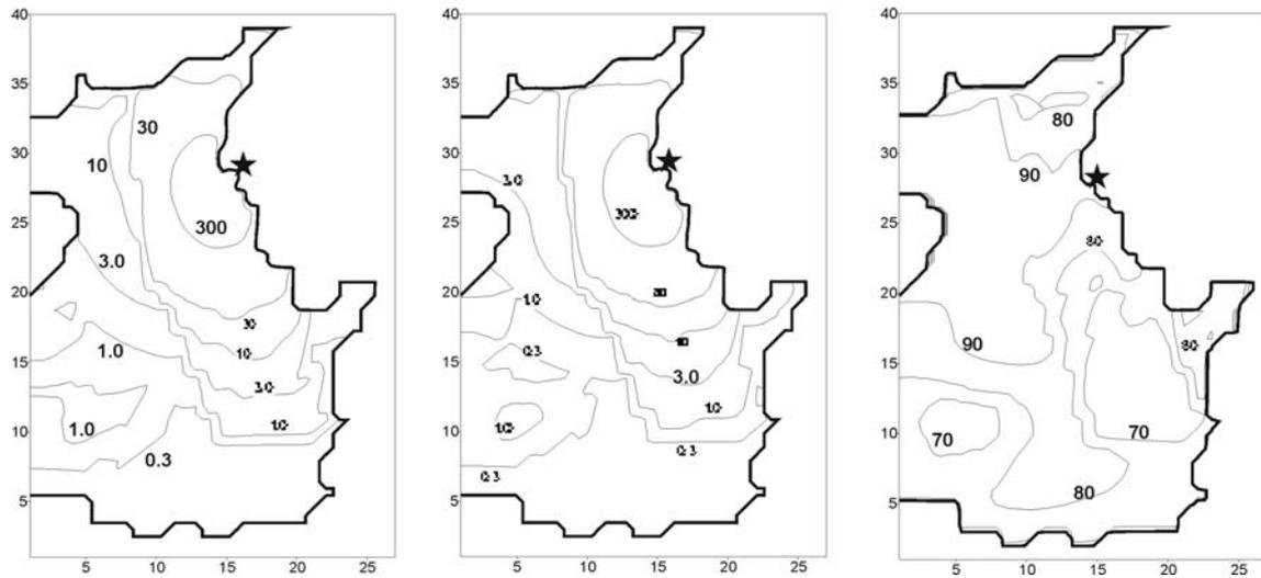
Figure 5.2. Examples of the computed distributions of  $^{239,240}\text{Pu}$  in bed sediments ( $\text{kBq/m}^2$ ) for year 1977 with the 1-step (left) and 2-step (centre) models. The star is Sellafield reprocessing plant. The map on the right is the computed fraction of reduced Pu in bed sediments (the same result with both models)
