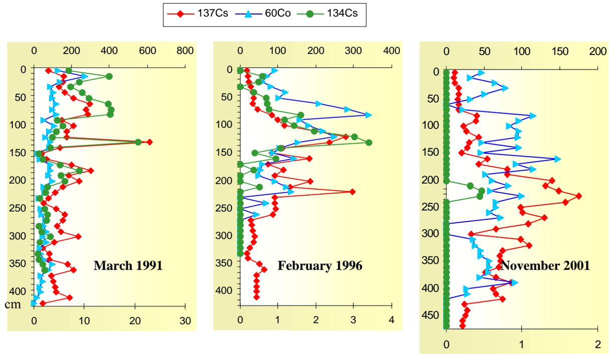
Figure 11: Vertical profiles of  $^{137}\text{Cs}$ ,  $^{134}\text{Cs}$  and  $^{60}\text{Co}$  (Bq kg<sup>-1</sup> dry weight) in long cores (>400cm) sampled at the Roustan station close to the Grand Rhône mouth in 1991, 1996 and 2001
