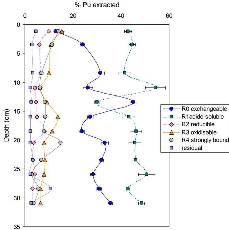
**Figure 2.** Sequential extraction of  $^{239,240}\text{Pu}$  from successive sediment horizons (core INT-010)
