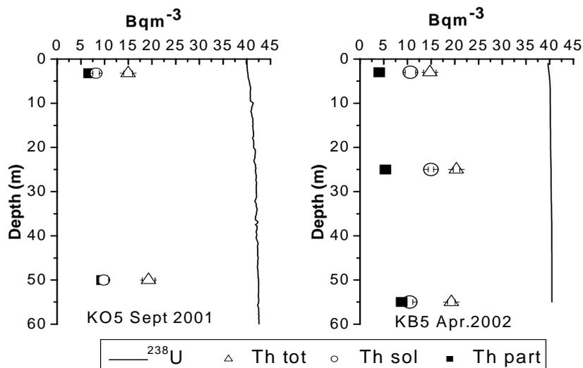
**Figure 6.** Vertical profiles of soluble and particulate  $^{234}\text{Th}$  in the water column of the inner Kongsfjord in summer (September 2001) and winter (April 2002).
