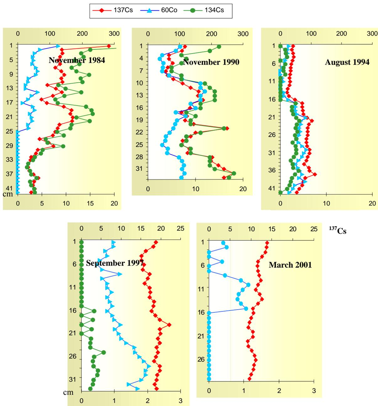
Figure 11 : Vertical profiles of  $^{137}\text{Cs}$ ,  $^{134}\text{Cs}$  and  $^{60}\text{Co}$  ( $\text{Bq kg}^{-1}$  dry weight) in cores sampled at the Roustan station close to the Grand Rhône mouth in 1984, 1990, 1994, 1997 and 2001. (Vertical scale in cm, notice the change of horizontal scale from 1997 onwards)
