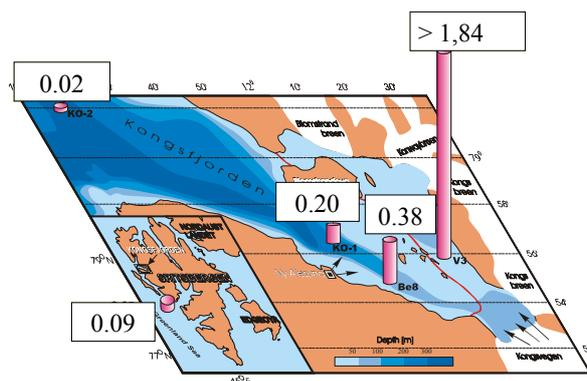
**Figure 7.** Sedimentation rates in Kongsfjord. ( $\text{g cm}^{-2} \text{ y}^{-1}$ )
