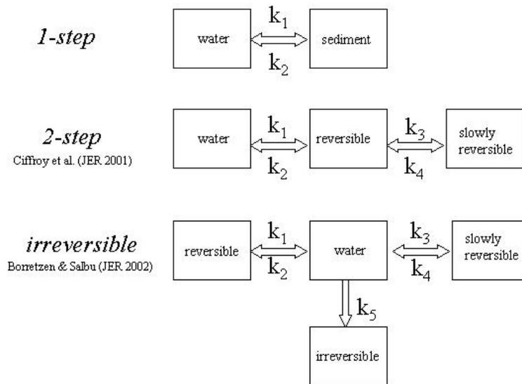
Figure 5.1. Kinetic models included in the hydrodynamic dispersion models
