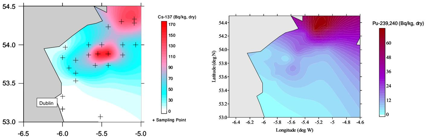
**Figure 2.** Distribution of  $^{137}\text{Cs}$  and  $^{239,240}\text{Pu}$  in Western Irish Sea Sediments
