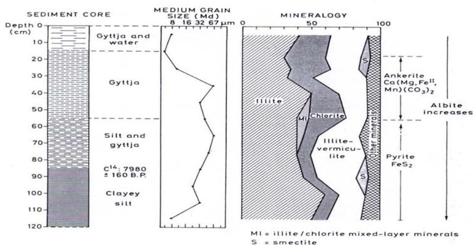
**Figure 11.** Vertical distribution of texture and mineralogical composition of sediments in Lake Rørholtfjord
