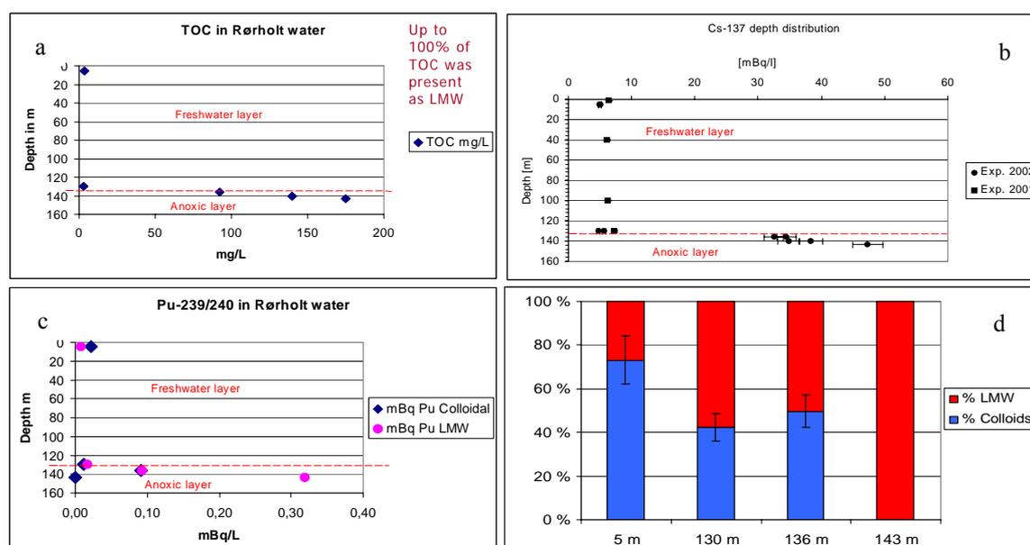
**Figure 10.** Vertical distribution of the concentration of a) total organic carbon, b) <sup>137</sup>Cs, c) <sup>239,240</sup>Pu in the water profile, and d) the speciation of <sup>239,240</sup>Pu in the waters.
