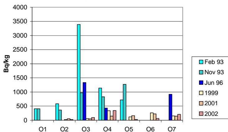
Figure 12.  $^{226}\text{Ra}$  in Odiel river sediments.
