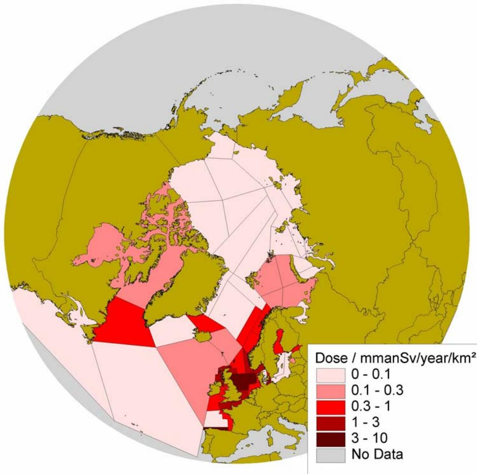
Figure 5.7. Collective dose rate after 10 years from different marine regions per 1 km<sup>2</sup> after a uniform deposition of <sup>137</sup>Cs at 1 kBq m<sup>-2</sup>
