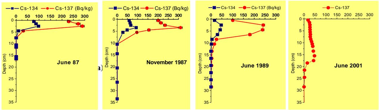
Fig. 18 - Vertical profiles of Cs isotopes at station 527, 1987 – 2001.
