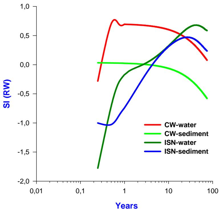
Figure 5.6. Local sensitivity analysis: relative dispersion of  $^{239}\text{Pu}$  in the Irish Sea regions versus relative sediment reworking rate
