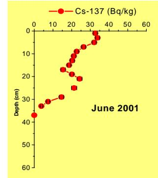
Fig. 20 - Vertical profiles of  $^{137}\text{Cs}$  and  $^{134}\text{Cs}$  at St. 567, in the inner Gulf of Trieste, 1987 (a), and 2001 (b).
