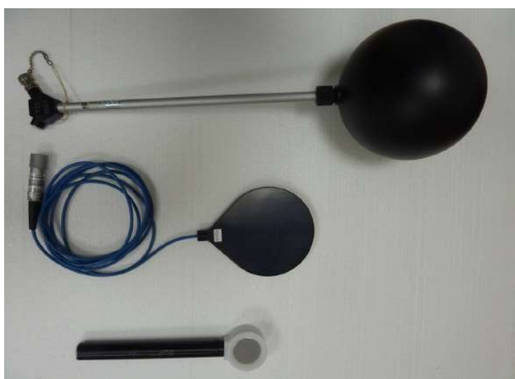
Dissemination of metrology traceability on national and international level; ionisation chambers from top to bottom: 1. LS-01 ensures the traceability for ^{137}\text{Cs} , ^{60}\text{Co} , ^{241}\text{Am} sources, and X-ray narrow spectra ;2. TW 34060 ensures traceability for RQR and RQA radiation qualities; 3. RC 06 M ensures traceability for RQR-M in RQA-M radiation qualities
