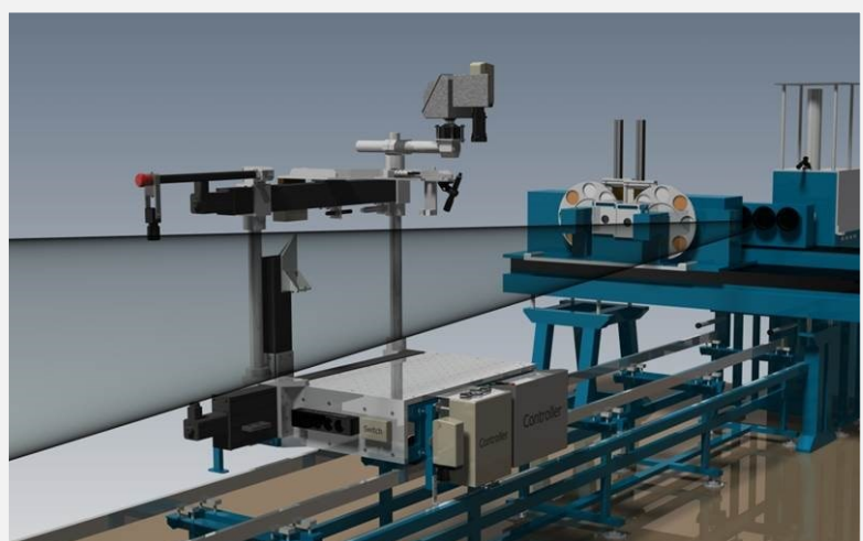
A CAD-drawing of the photon irradiation set-up. The field generated by one of the ^{137}\text{Cs} sources is displayed. The X-Ray tubes with the different filter options mounted on the two wheels have been moved into the parking position
