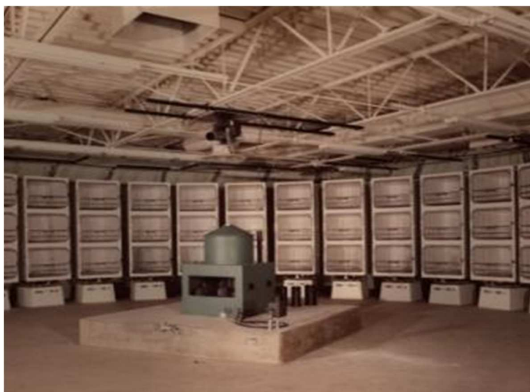
Janus irradiator configuration surrounded with animal cages
