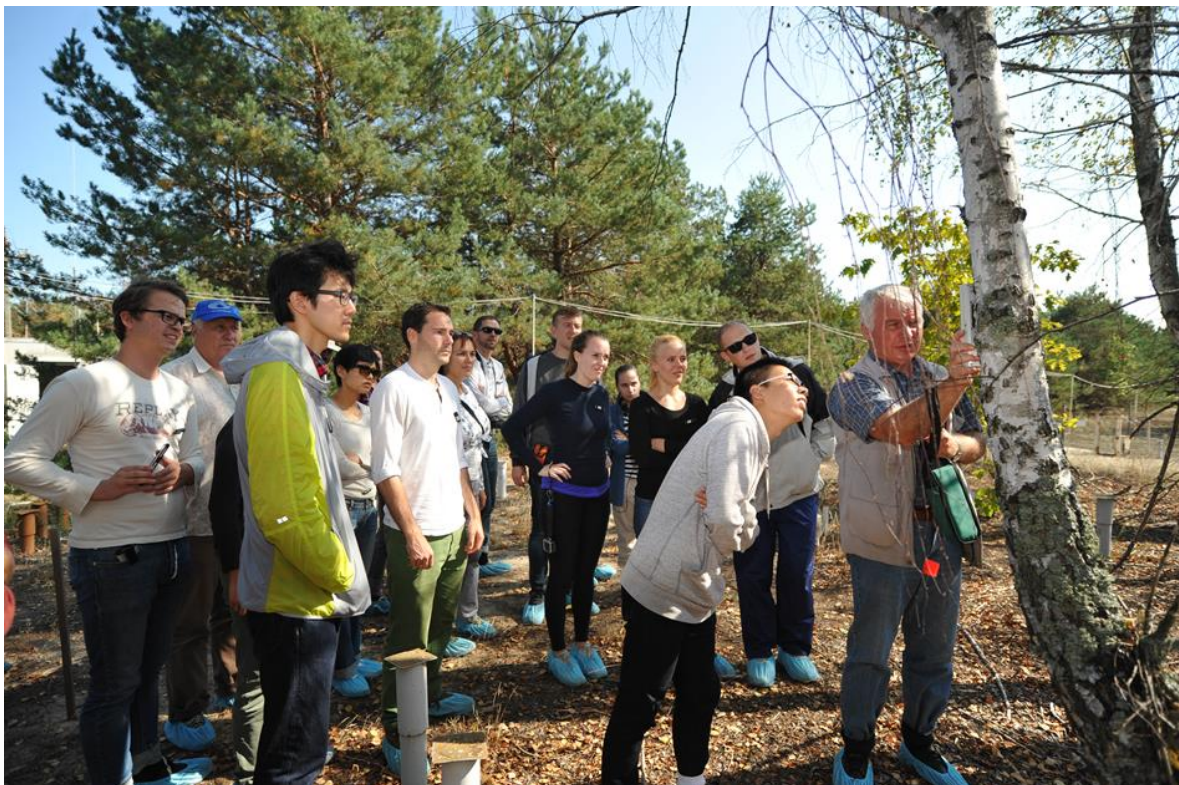
Picture 2 Measuring dose from contaminated trees (Photo: V. Kasparov)
