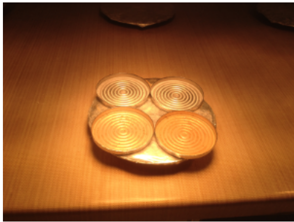
Figure 1.- Evaporation of samples in planchets under infrared lamps.
